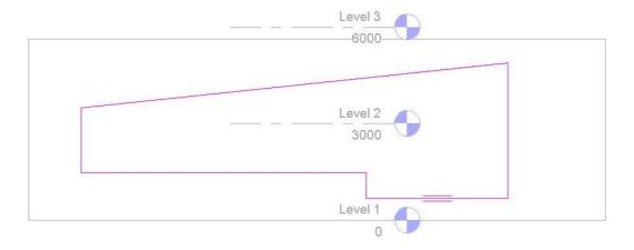
Click on "Beam Direction" (left pane) and click on the bottom line to say where you want the beams to start and in what direction.
